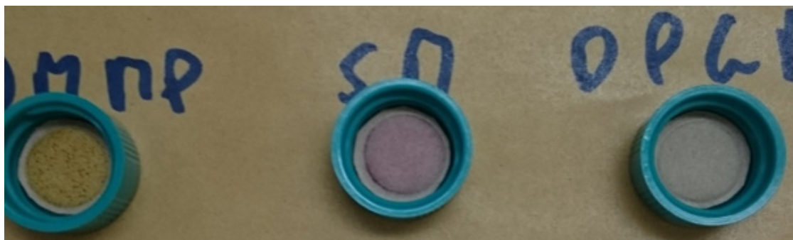
Figure 3c: Paper detectors placed in RT 70 mm over drops of liquid DMMP; SM; DPGM simulants after 168 hours.
