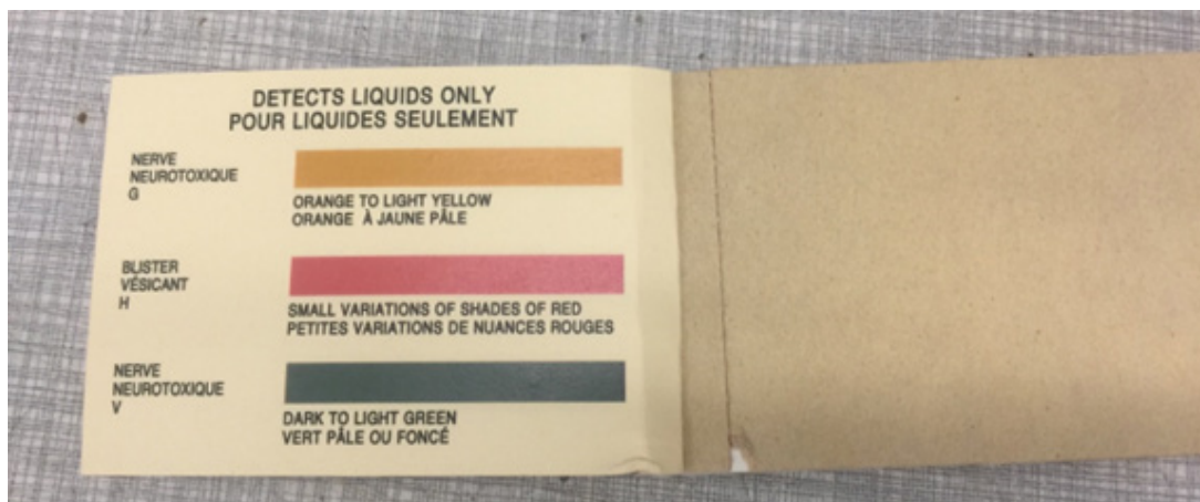
Figure 2: Brown self-sticking paper colorimetric detector (right) changing rapidly colour after contact with liquid CWA (left).
