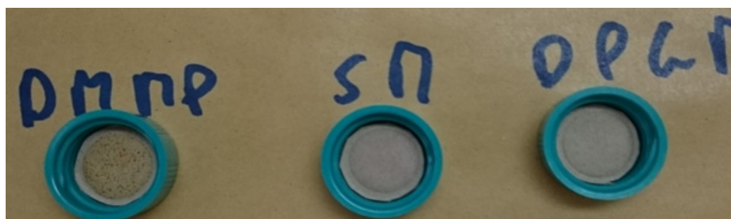
Figure 3b: Paper detectors placed in RT 70 mm over drops of liquid DMMP; SM; DPGM simulants after 48 hours.
