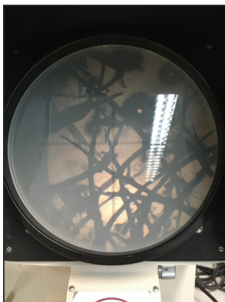
Figure 1: The A4 copy paper sample Q Connect consisted of chemical pulp i.e. cellulose, since the color of the stained specimen in the optical microscope was dark bluish-violet. The microscope used was a projection optical microscope SDL S.N., 232431, 220V, 60W, S1, with a round screen and no binoculars, and with a magnification of x10/0.2 to x20/0.4.
