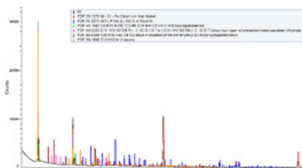
Figure 9: XRD for phosphating coatings of the samples at 40 °C using the mobile device method.
