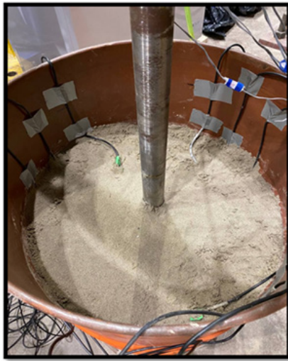
Figure 3: Model soil preparation and instrumentation.
