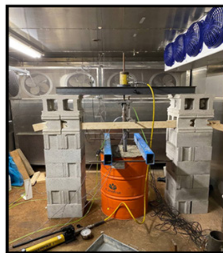
Figure 2: a) Schematic view of experimental setup, b) A view of the model pile and the soil container (barrel) used in this experiment.
