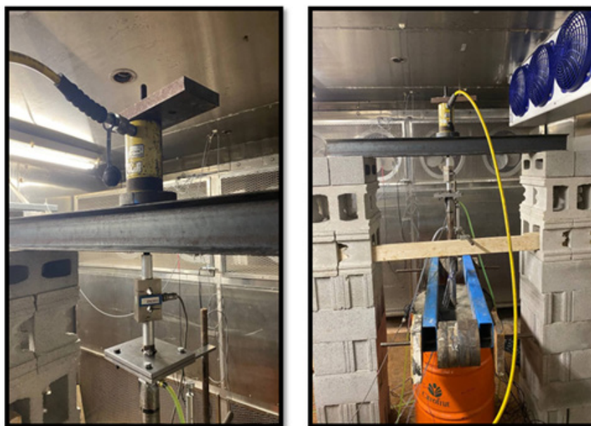
Figure 11: Pile pull-out testing assembly and setup.
