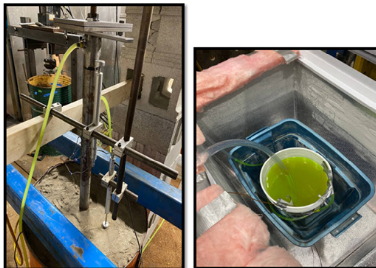
Figure 7: The freezer and Antifreeze as source of cold temperature.
