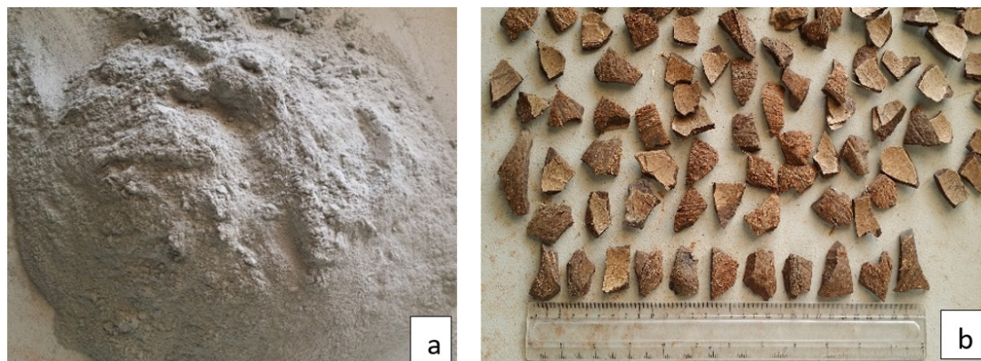
Figure 1: Materials for concrete production: (a) metakaolin used as cement, (b) coconut shells used as coarse aggregate.
