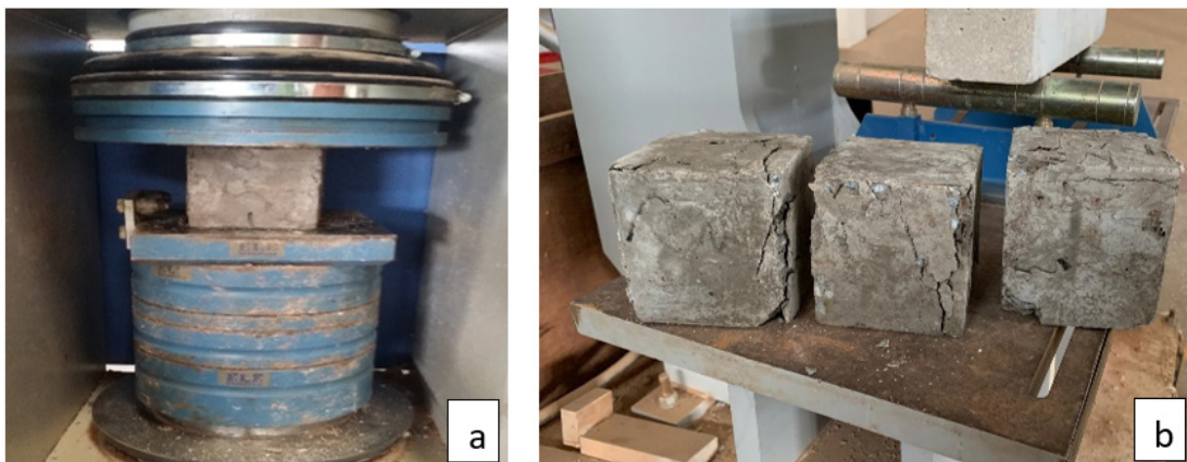
Figure 4: Compressive test process: (a) compressive test setup, (b) failed specimen.
