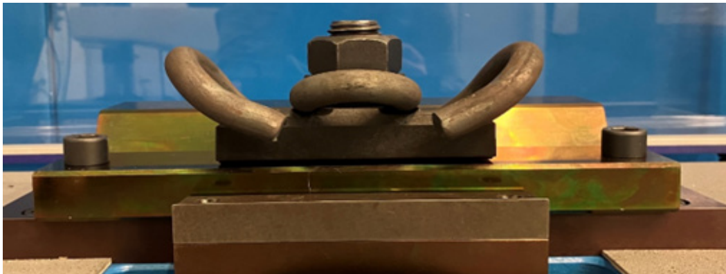
Figure 6: SKL14 fatigue test setup [1].
