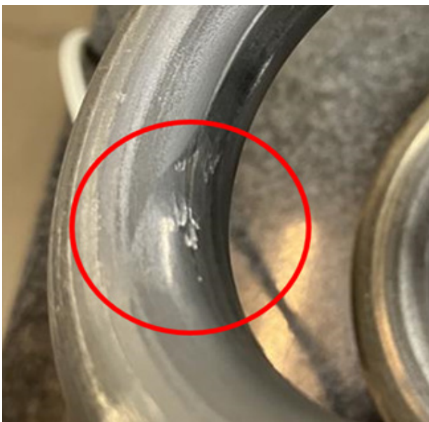
Figure 4: Bending marks on the surface of clip [1].
