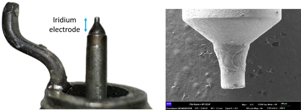
Figure 1: Left: Image of an optical microscopy of the tip of a spark plug where the Iridium electrode is located. Right: SEM image of the Iridium tip.
