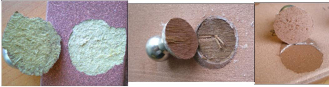
**Figure 8:** Images of the copper coating adhesion results to MDF (top), mahogany wood and terracotta tiles (bottom).
