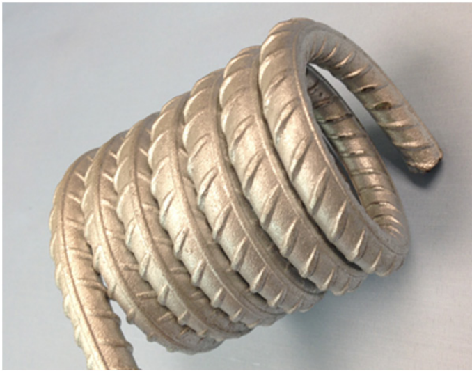
Figure 1: Continuous Galvanized Rebar exhibits excellent formability.
