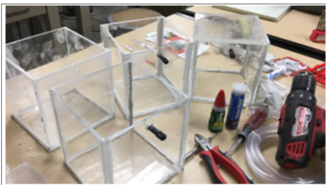
Figure 2: Assembled cubicle tanks with sharp and round edged orifice
