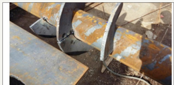
Figure 1: Screw defects - tears.
