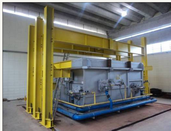
Figure 2: Detail of the furnace of test for horizontal structural elements, built at EESC/USP, Brazil.
