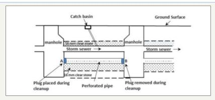
Figure 1: Schematic of Double Pipe Technology Scenario.
