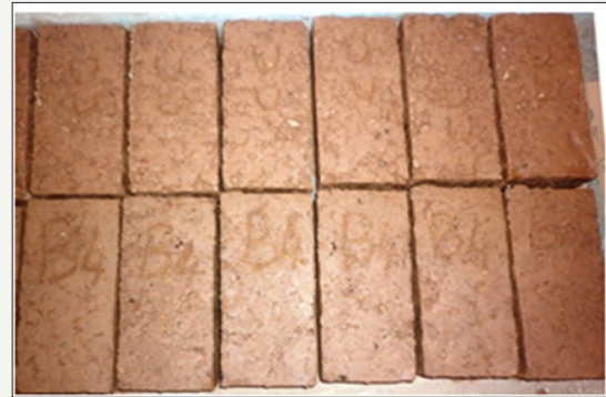
Figure 2: Freshly Moulded Earth Bricks.
