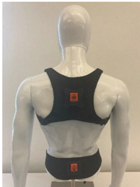
Figure 1: IMU sensor configuration for Lumbar Spine Motion Assessment
