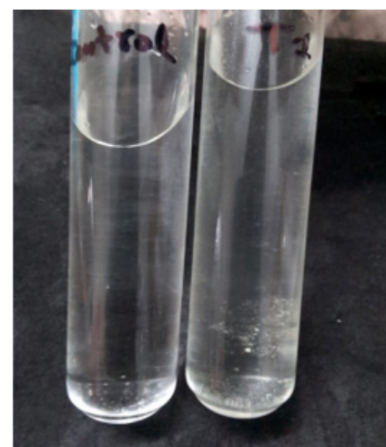
Figure 2: Calcite precipitation by T1 without filtration.
