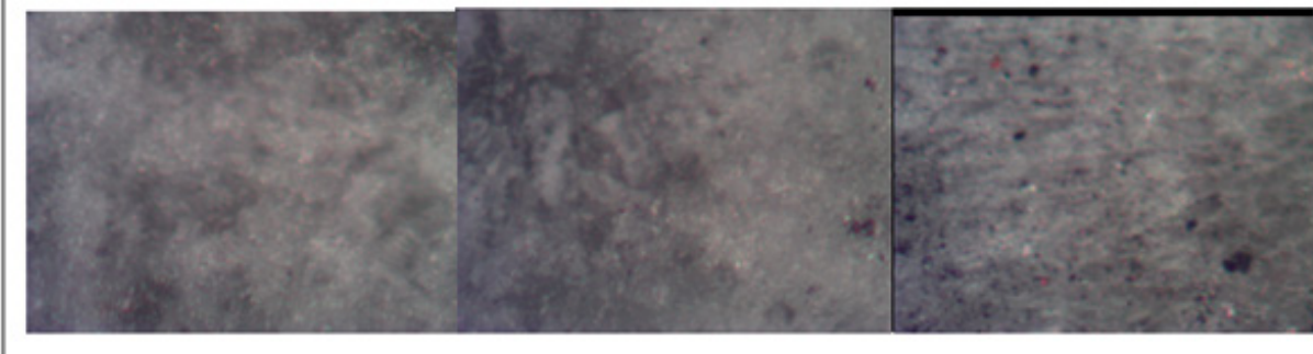
Figure 5: Pictures of slab 6 immersed into HCl solution at 0, 8 and 43 days.
