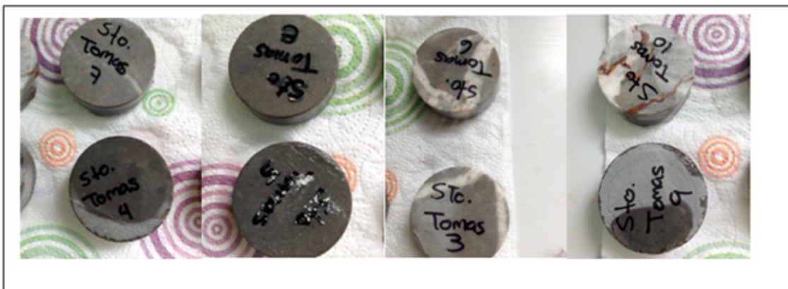
Figure 4: Picture of the slab top immersed into HCl (3,6), H 2 SO 4 (5,8), CaCO 3 (4,7) and H 2 O (9, 10), experimental time 36 days.
