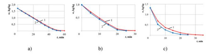
Figure 2: Curves for drying textiles
