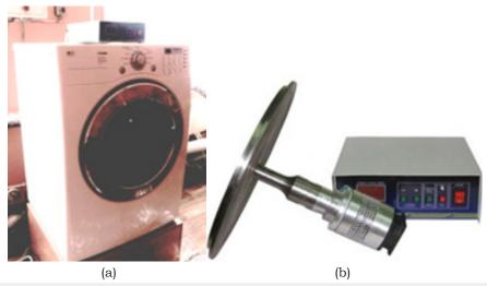
Figure 1: Photograph of a drum dryer with an ultrasonic apparatus.
