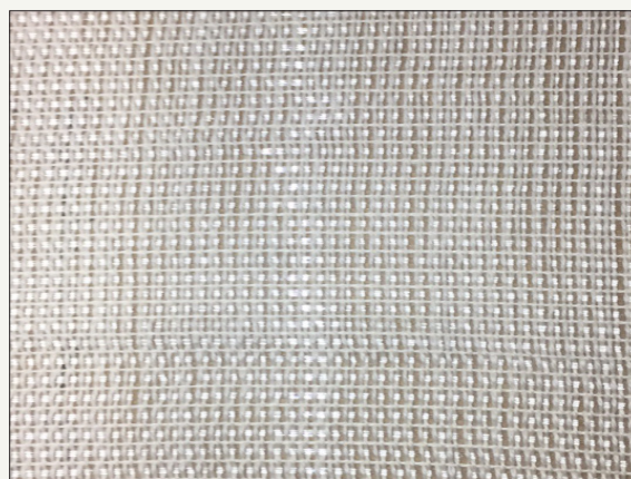
Figure 4b : The fabric with POF as the weft yarns and cotton as the warps produced.
