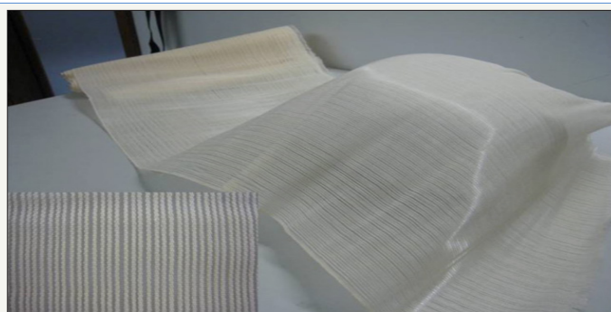
Figure 1: Photograph of woven fabrics produced from cotton yarns and POF of diameter 250µm [13].
