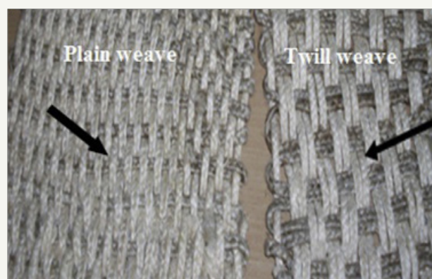
Figure 6: The weaving pattern used Alavudeen et al. [20].
