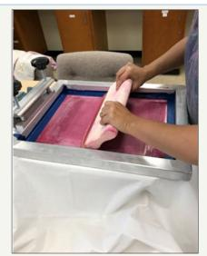
**Figure 7:** The fabric printed with squeegee using the prepared screen.
