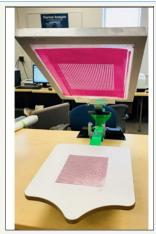
Figure 6: Screen printing machine used for the process.
