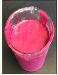
**Figure 5:** The ready printing ink using cochineal pigment and the thickener.
