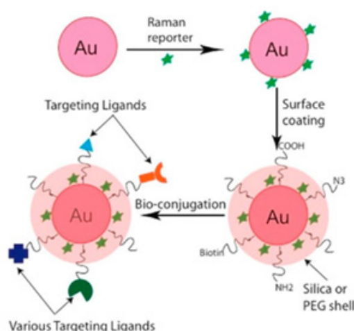
Figure 5: Overview for the design of a SERS tag formed by a Raman reporter, plasmonic core, targeting ligands, and colloidal stability coating. Adapted with permission from [52].
