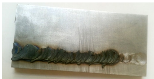
Figure 4: A typical coating by friction surfacing process of A60 steel on X48 steel.
