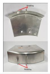
**Figure 5:** A formed specimen sample with wrinkling defect (material: AA2024-W, thickness: 1.27mm, contour radius: 125mm, flange length: 40mm).
