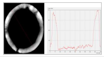
Figure 9: Cross-section of the pipe and its profile along the line running through the center of the pipe.
