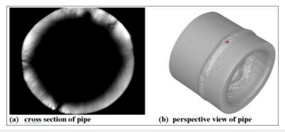
Figure 7: Cross section and a promising view of the reconstructed pipe image.
