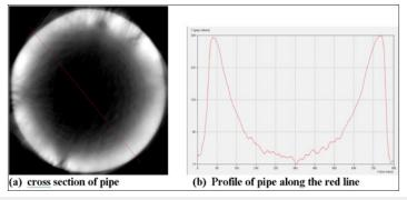
Figure 8: Cross section of the pipe and its profile along the line running through its center.
