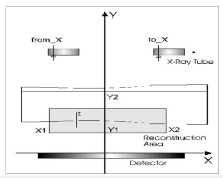
Figure 1: Scan geometry for reconstruction longitudinal profile pipes.
