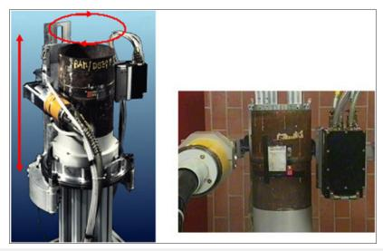
Figure 2: Mechanized tomographic radiometric system.
