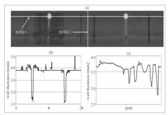
**Figure 5:** Reconstruction results: (a) gray value representation of inner pipe surface together with pipe profile along the circle, thickness profile 1 and profile 2 along pipe axis shown in (b) and (c), respectively.
