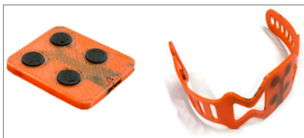
Figure 10: Photograph of 3D-Printed EMG electrodes using flexible conductive filaments (TPU/Carbon black based).
