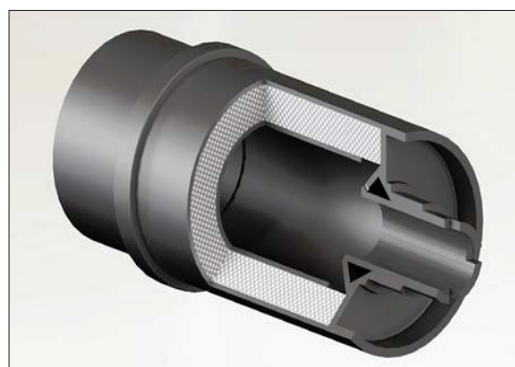
Figure 8: Optimized H13 rotor shaft with lattice structures for lightweight design optimization.
