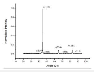
**Figure 6:** X-ray Diffraction profile of ADI from Batch A.
