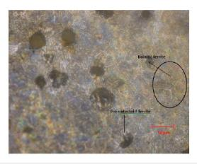
**Figure 7a:** Microstructure of step-up austenitized ADI (Batch H).
