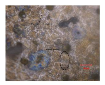
**Figure 4a:** Microstructure of step up austenitized ADI (Batch A).
