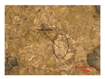
**Figure 4c:** Microstructure of conventionally processed ADI (Batch C).
