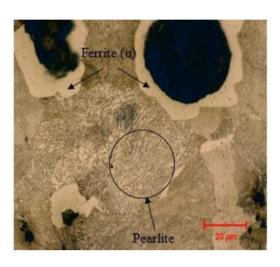
Figure 3: Optical microstructure of the as-cast microstructure of ductile cast iron.
