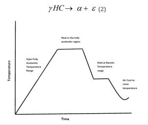
**Figure 1:** Heat treatment cycle for conventionally processed ADI.
