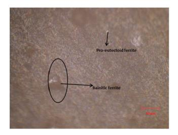
**Figure 4d:** Microstructure of step up processed ADI (Batch G).
