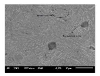
**Figure 8b:** SEM microstructure of step-up austenitized ADI austempered (Batch H).
