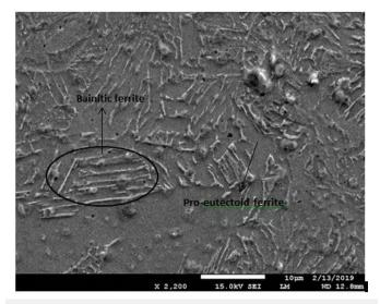
**Figure 8C:** SEM microstructure of step-up austenitized ADI austempered (Batch I).
