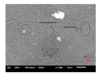
**Figure 8a:** SEM microstructure of step-up austenitized ADI austempered (Batch A).
