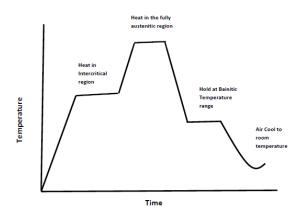
**Figure 2:** Schematic of the proposed heat treatment Cycle for ADI processed via step up austenitization.
