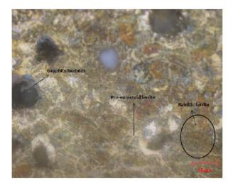
**Figure 7b:** Microstructure of step-up austenitized ADI (Batch I).
