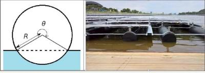
Figure 2: Example of a floating plant with detail of the pipes buoyancy.
