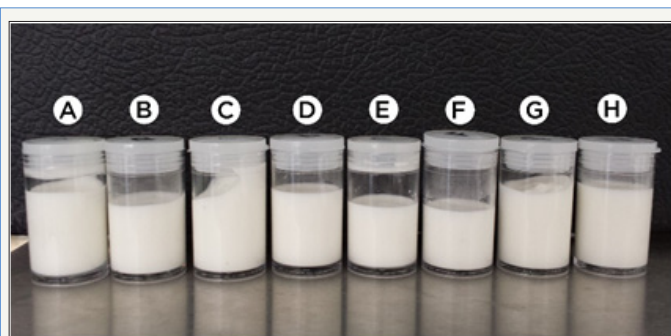
Figure 1: Appearance of canola-based emulsions prepared with 3 or 5% (w/v) surfactants Tween® 60 (A, C, E, and G) or Tween® 85 (B, D, F, and H).
