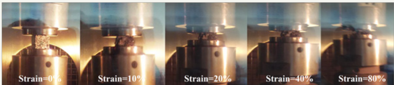
Figure 4: Deformation mechanism of Al-Si7Mg Al alloy foam with 10wt% SiC particles.
