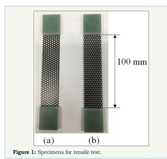
Tensile tests were carried out at 100 K, room temperature and 373 K in thermostatic chamber (Figure 2). These temperature environments were achieved by a PID controller with a liquid nitrogen sprayer and a heater. The tensile testing machine (AG-100 KNX Shimadzu Co. Ltd., Japan) was operated at a crosshead
