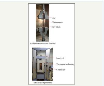
Figure 2: Experimental set-up of tensile test.
