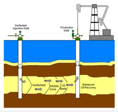
Figure 1: Schematic of a surfactant-based flooding process applied to a petroleum field.
