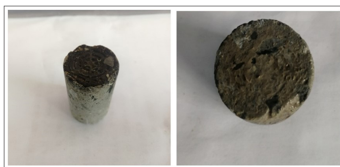
Figure 6: Natural volcanic rock core 1-1 flow blockage after experiment.
