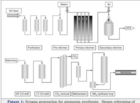
**Figure 1:** Syngas generation for ammonia synthesis: Steam reforming of natural gas, HTS converter unit, LTS converter unit [10].
