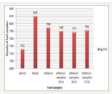
Figure 3: Density of petrol, diesel, ethanol, ethanol-camphor (9:1), ethanol-camphor (8:2) and ethanol-camphor (7:3) at 35 °C.
