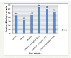
**Figure 1:** Duration of burning of petrol, diesel, ethanol, ethanol-camphor (9:1), ethanol-camphor (8:2) and ethanol-camphor (7:3) in open flame system.
