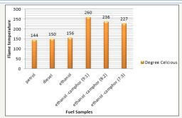
**Figure 2:** Flame temperature of petrol, diesel, ethanol, ethanol-camphor (9:1), ethanol-camphor (8:2) and ethanol-camphor (7:3) in open flame system.
