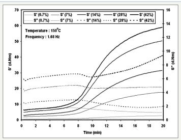
Figure 10: Cure torques against time at different strains.
