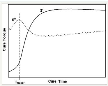
Figure 3: Typical torque responses resulting from RPA cure test.
