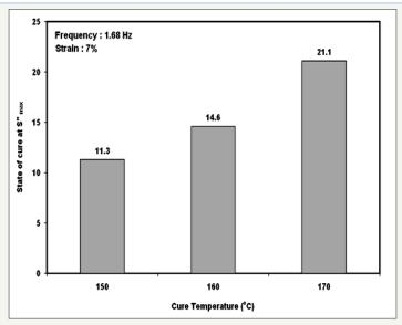
**Figure 6:** State of cure at  $S_{max}$  for different cure temperatures.
