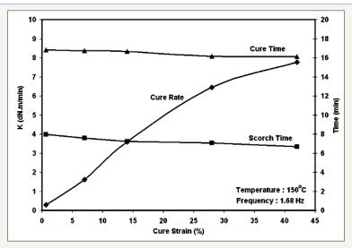
Figure 11: Cure characteristics versus cure strain.
