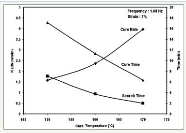
Figure 5: Cure characteristics at different temperatures.
