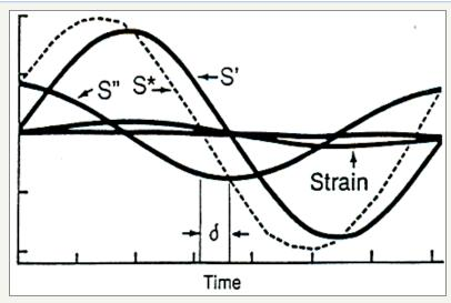
Figure 2: Applied strain and torque responses in RPA.
