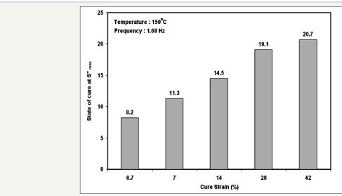
Figure 12: State of cure at  $S"_{\mbox{\tiny max}}$  for different cure strains.
