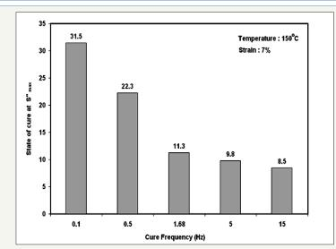
Figure 9: Changes in the state of cure at  $S^{"}_{\ \ max}$  with the cure frequency.
