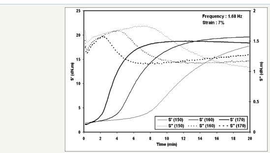
Figure 4: Influence of temperature on the cure torque curves.
