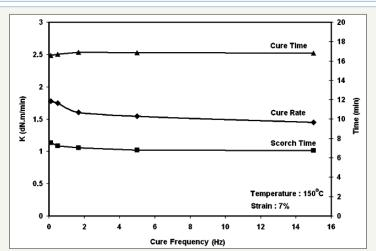
Figure 8: Cure characteristics against the cure frequency.
