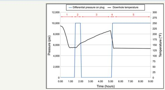
Figure 1: Simulated temperature and pressure response during hydraulic fracturing.
