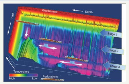
Figure 3: Measured temperature profile from three stages of hydraulic fracturing [10].
