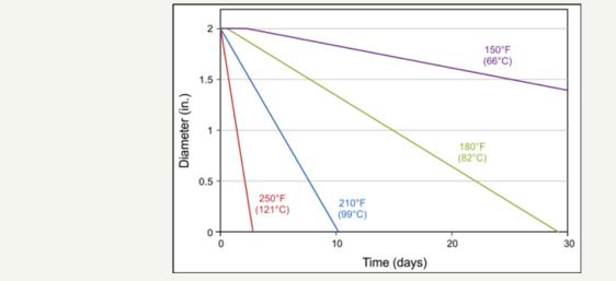
Figure 8: Temperature sensitivity of the degradation of PGA plastic [18].
