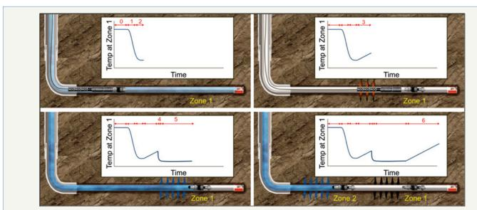
Figure 10: Down hole temperature, such as at the frac plug for Zone 1, varies during the hydraulic fracturing process.
