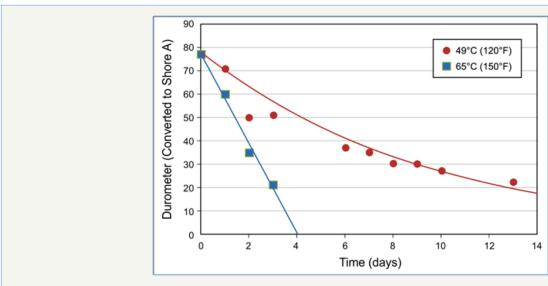
Figure 7: Degradation of low-temperature elements at 65 and 49 °C (150 and 120 °F).
