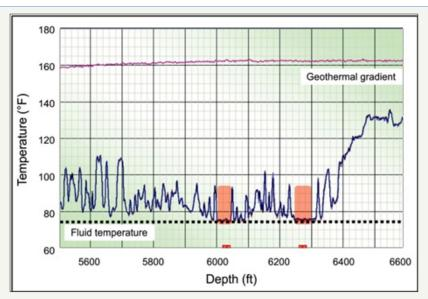
Figure 2: Events during a simulated hydraulic fracturing stimulation [10].
