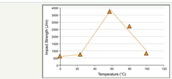
Figure 9: Temperature sensitivity of the impact strength of PGA plastic [18].
