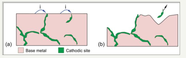
**Figure 4:** Schematic presentation of the degradation between the base metal and the cathodic phase; (a) Micro-Galvanic corrosion of base metal; (b) intermediate corrosion shape.
