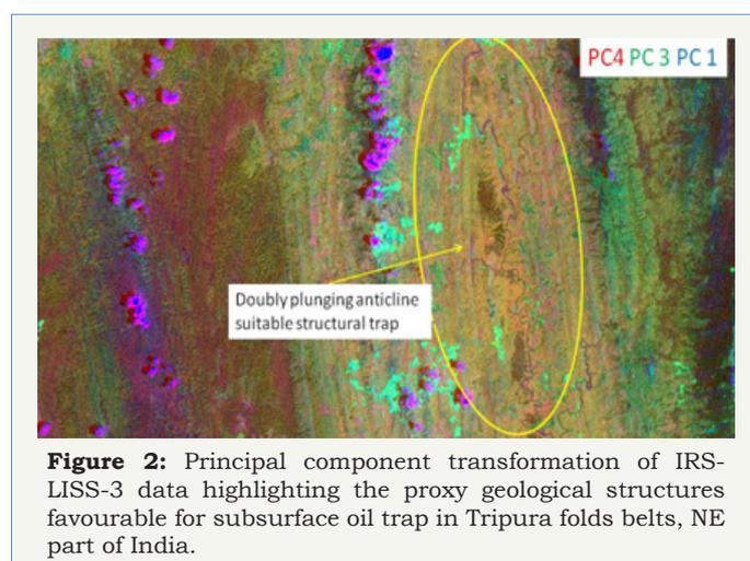
**Figure 2:** Principal component transformation of IRS-LISS-3 data highlighting the proxy geological structures favourable for subsurface oil trap in Tripura folds belts, NE part of India.
