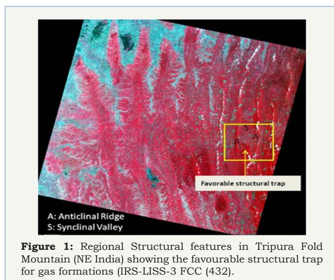
**Figure 1:** Regional Structural features in Tripura Fold Mountain (NE India) showing the favourable structural trap for gas formations (IRS-LISS-3 FCC (432)).
