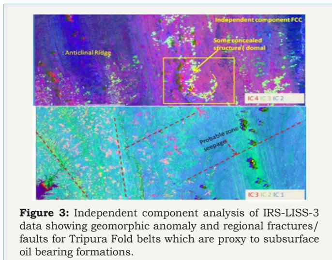
**Figure 3:** Independent component analysis of IRS-LISS-3 data showing geomorphic anomaly and regional fractures/faults for Tripura Fold belts which are proxy to subsurface oil bearing formations.
