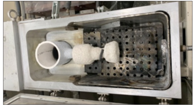
Figure 2: Vacuum centrifugal casting apparatus for TiAl alloy.
