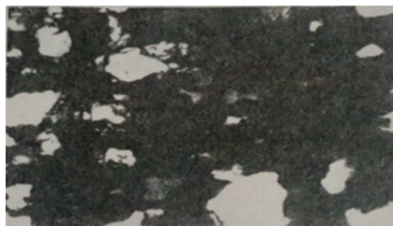
Figure 3b: Stretching of quartz and opaques within manganiferous quartzose band. X10, Tirodi mines.
