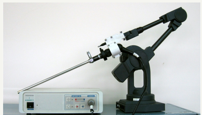
Figure 4: 3D-digitazer Microscribe G2 with laparoscope.
