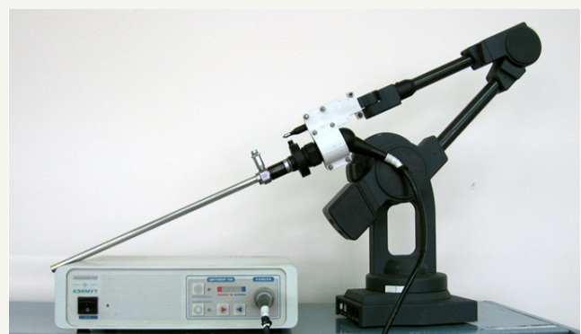
Figure 4: 3D-digitazer Microscribe G2 with laparoscope.
