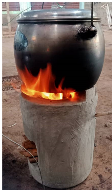
Figure 6: Flame visualization of 1 hole of SA stove.
