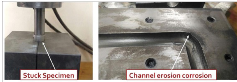
Figure 7: Results of poor lubrication.
