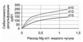
Figure 1: Dependence of cast iron desulfurization from Mg consumption and diameter of powder wire.
