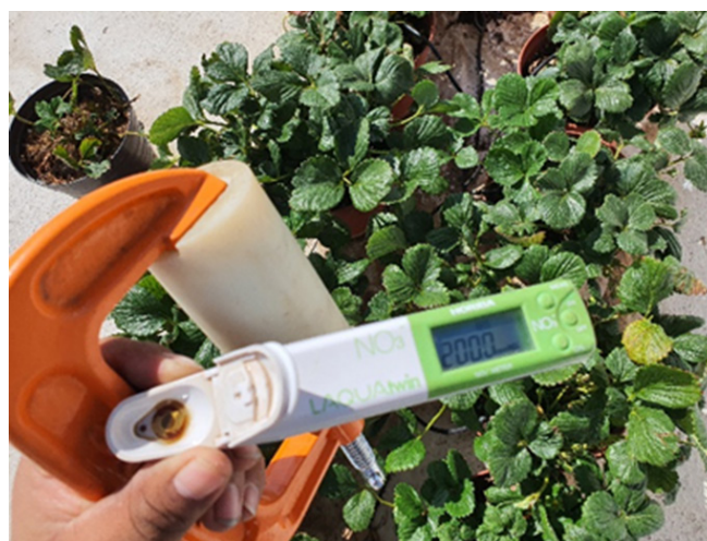
Figure 1: Extraction of the nitrate sap using a mechanical press.
