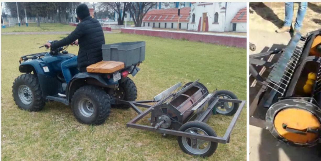
Figure 2: Fruit picker in the back of the cuatrimotor showing some fruits inside the cylinder.
