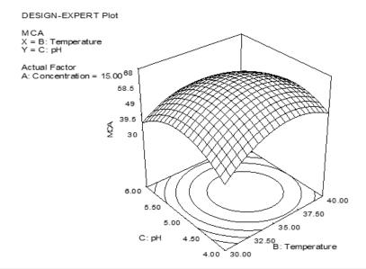
**Figure 2:** Response surface plot for MCA as a function of pH and temperature at fixed enzyme concentration of 15μL/mL of milk.
