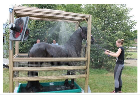
Figure 1: An example of a single Equine Cooling Unit (ECU) in operation.
