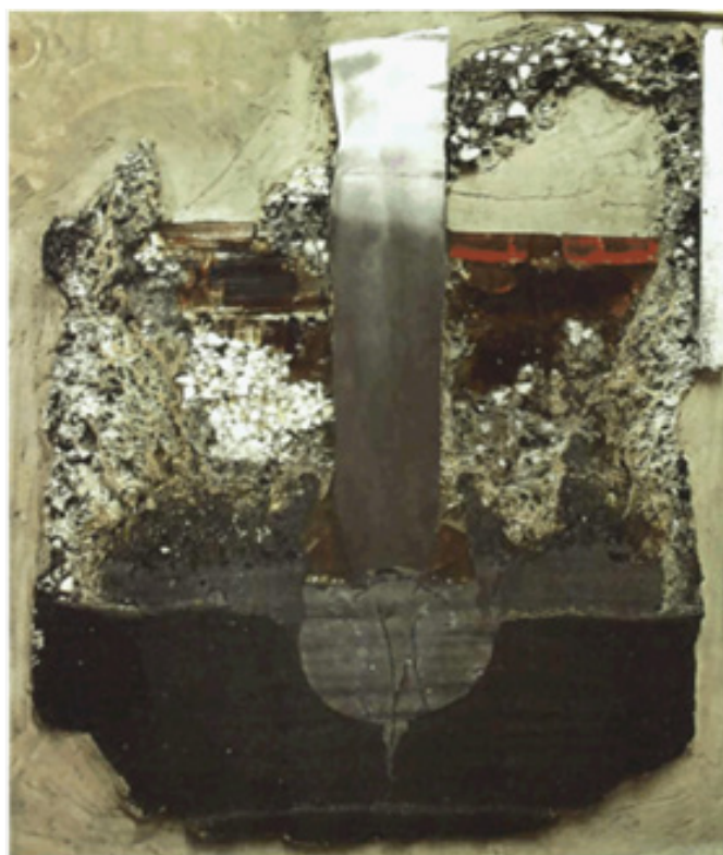
Figure 1: Recreated cross section with various material zones defined by color (left) and a picture of the cross section (right) from Myrhaug's pilot scale excavation, used with permission from [3].
