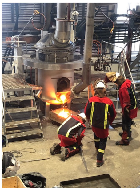
Figure 4: Photo taken by Haley Hoover of furnace tapping during pilot scale furnace operations.
