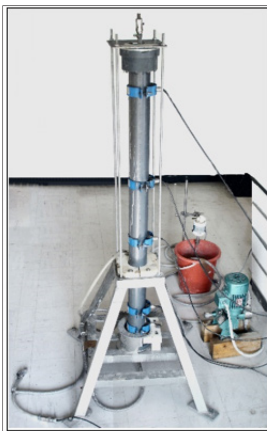
Figure 1: Laboratory equipment for penetrability evaluation [8-14].
